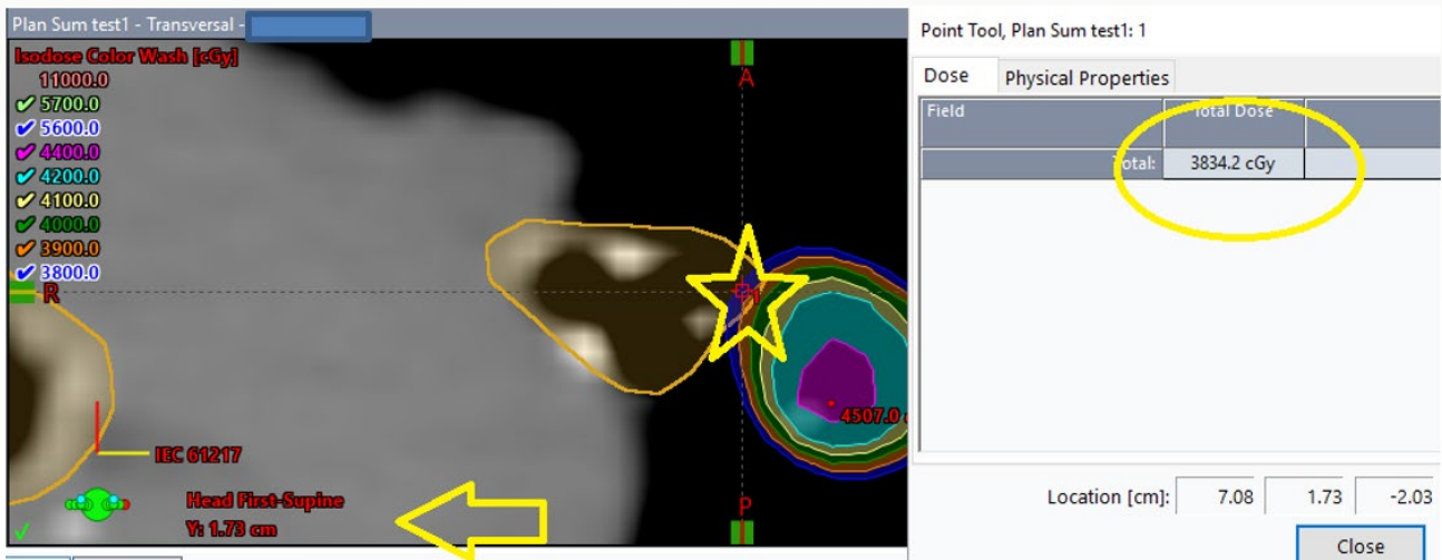
Figure 1: Plan sum dose cloud display, showing the TrachBronchTree contour extending into the 3900 cGy dose cloud, but a reported maximum dose of less than 3900 cGy
