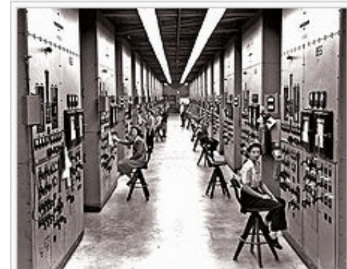
Employees of the Manhattan Project operating calutron control panels at Y-12, in a US government photo by Ed Westcott .
