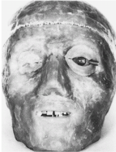
Fig. 2. The phantom used in the radiation studies was a human skull covered with a mixture of paraffin and beeswax and filled with bolus. Provision was made in the plastic eye to place a small Baldwin-Farmer Condenser ionization chamber in the position of the lens. Reproduced by permission from Merriam, G. R., Jr., and Focht, E. F.: A clinical study of radiation cataracts and the relationship of dose. Am. J. Roentgenol. 77:759-85, 1957.
