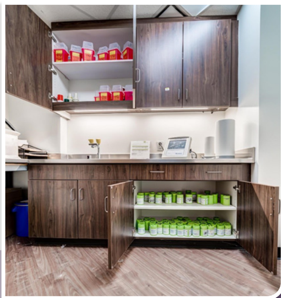
Figure 2: A cabinet for storing used vials in their lead shields (lower cabinet) and a cabinet to store radioactive waste containers (used needles, alcohol wipes, gloves, etc.). A large waste drum is available as needed.
